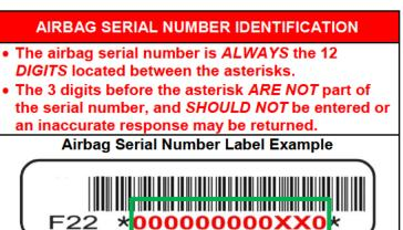
The AIRBAG serial number MUST be recorded prior to replacement.
