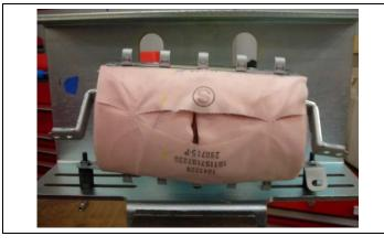
c) Mount the airbag to the mouting bracket as shown.
