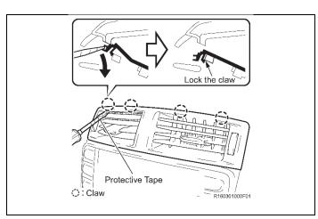
Removing the No. 3 air register
