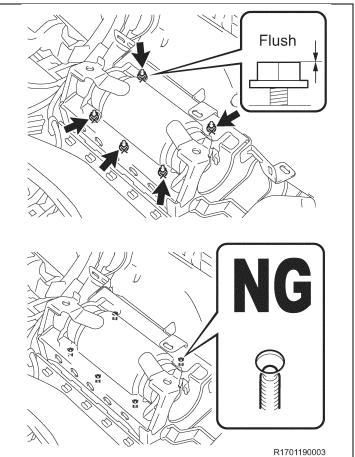
d) Loosen the 5 nuts until each nut is flush with the top of the stud as shown.
