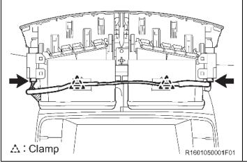
Disconnect the connectors and clamps from the register.
