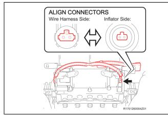
m) Connect the connector and the secondary lock.
