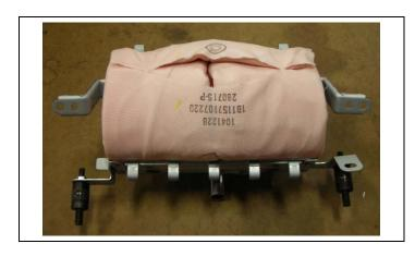
b) Mount the adaptors (579943-3R3) to the airbag as shown.
