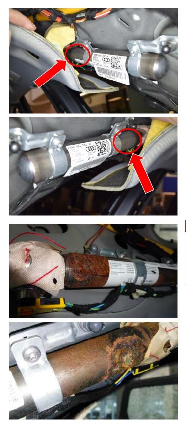
Gently lower the headliner on the right and left sides to inspect the head curtain inflators <arrows> for corrosion. Pay particular attention to the areas that were covered by the foam block.
