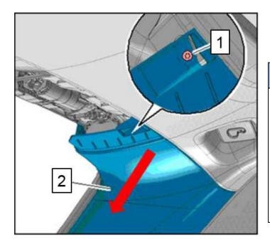
• Remove the expanding clip rivet <1> by placing the pry lever -80-200- between the headliner and the sheet metal/body. Repeat for both sides.
