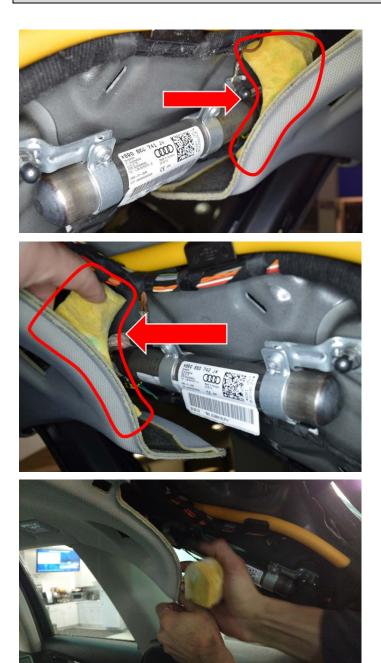
Remove and discard the foam padding from • the headliner on the right and left side by gripping the foam padding with the fingers and peel the foam away from the headliner.
