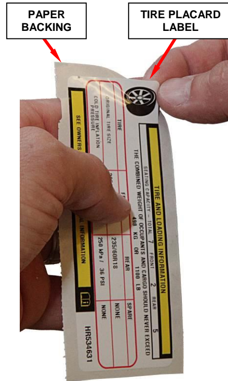
Figure 5 – Remove Tire Placard Label From Paper Backing
