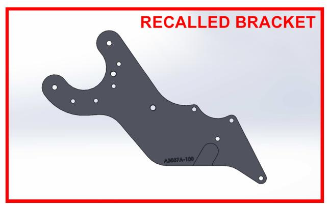
If you have one of the vehicles listed above, a visual inspection will easily identify whether you have a kit or system covered by this recall. The replacement part can be visually identified by the addition of an unused scribe hole on the front (forward) facing side of the new replacement bracket (See top two illustrations above, outlined in green).
