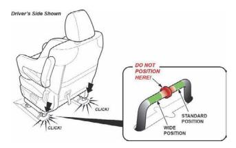
If despite the risks you choose to tip the entire second row seat forward to access the third row, make sure the seat is in the standard or wide position when lowering and latching the seat.
