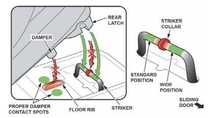
Check that the seat is latched by rocking the seat back and forth, trying to tilt it forward, and make sure both the inner and outer latches are locked and the front seat hooks are under the front strikers.
