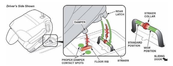
4. Press down on the rear part of the seat to set both rear latches. The latches click as they engage the floor strikers.
