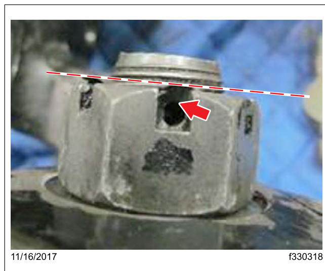
Fig. 7, Good Cotter Pin Hole Position
