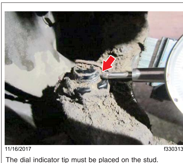
Fig. 2, Dial Indicator Tip Positioning
