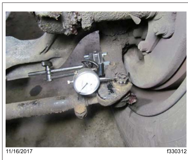
Fig. 1, Dial Indicator Mounting Position
