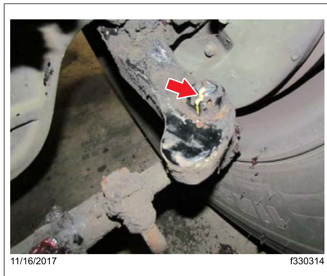
Fig. 3, Paint Mark to Identify Nut Rotation
