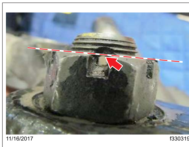
Fig. 8, Cotter Pin Hole at Maximum Height
