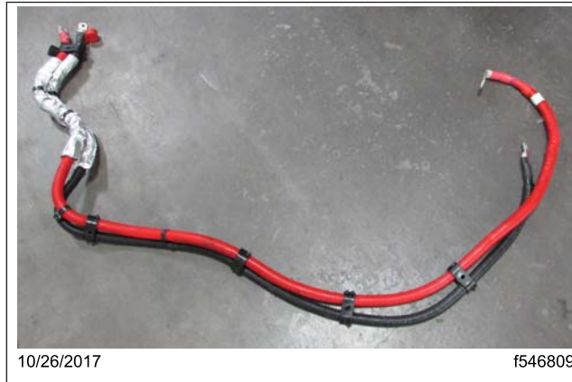
Fig. 4, Positive and Negative Battery Cables Removed
