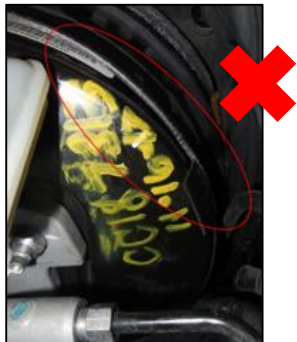
VIN/date written on the face of the brake booster instead of the top.
