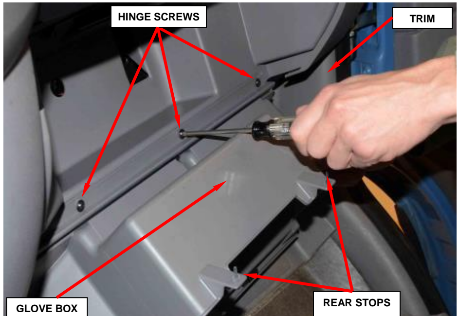
Figure 3 – Glove Box Hinge Screws
