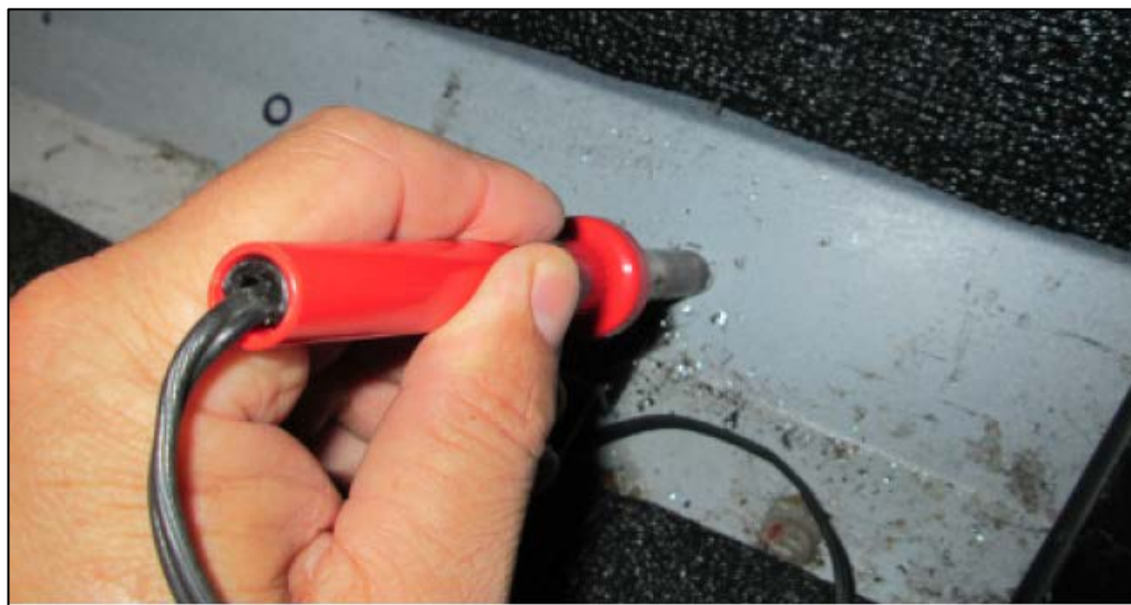
Figure 12: Removing Davenport Insulation
