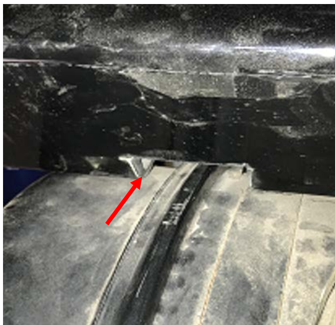
Figure 10: Notch for air filter canister cover
