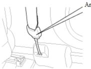
Anchor pretensioner connection to front seat belt linkage
