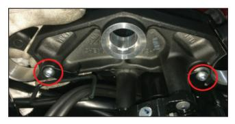
11. Remove 2 Torx® bolts. Cut the cable tie holding the harness and then unplug the connector. Remove the main-switch sub-assembly.
