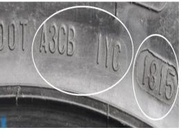
Tires made for use in the United States are required to have the DOT serial number and date located on one sidewall of the tire near the rim. The sample shows a tire manufactured during the 18<sup>th</sup> week of 2015.
