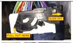
e) Slide the Connector Locking Arm off the connector by first pulling outward at the rear of the Arm on both sides, about 1/4" (6mm). This should be just enough for the slots on the Primary Locking Arm to clear the pins on the connector.
