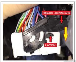
Slide the Connector Locking Arm off the connector by first pulling outward at the rear of the Arm on both sides, about 1/4" (6mm). This should be just enough for the slots on the Primary Locking Arm to clear the pins on the connector.
