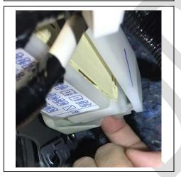
e) In the rear lower right corner of the JB is another release. Use your finger to pull out on the release tab and separate the bracket from the JB.
