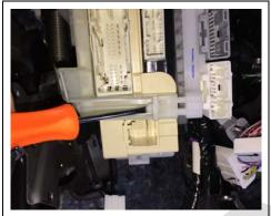
d) Attached on the right side of the JB is a bracket that holds additional connectors. Use a small screwdriver and release the locking tab in the front lower right corner of the JB.
