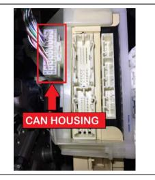
c) Pull the CAN Communication connector housing toward you and separate it from the JB. DO NOT pull by the wires.
