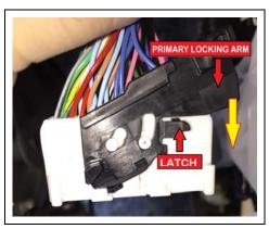
d) Fold the Connector Locking Arm to the locked position by first releasing the latch on both sides and then pivoting the arm to the locked position.
