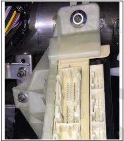
g) Remove the two nuts and lower the JB.
