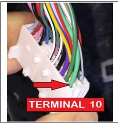
j) Turn the connector around to view the wire side. Locate the wire that is plugged into terminal 10. It will be a light green color.
