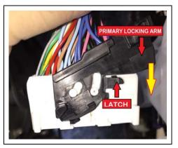
d) Fold the Connector Locking Arm to the locked position by first releasing the latch on both sides and then pivoting the arm to the locked position.
