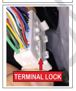
f) Unlock the secondary terminal lock by using a very small pick or screwdriver. Pry up at both ends until the secondary terminal lock has popped up about 1/16" (2mm)
