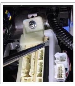
f) In the upper right corner of the JB is an additional release. Use a screwdriver to separate the bracket from the JB.
