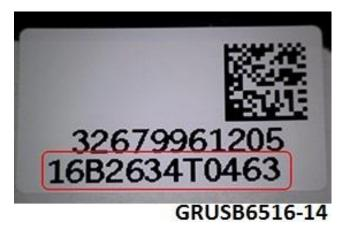
Before installing the replacement part, the new air bag module's serial number must be documented by the technician on the repair order so it can also be entered into the warranty claim's comment section.
