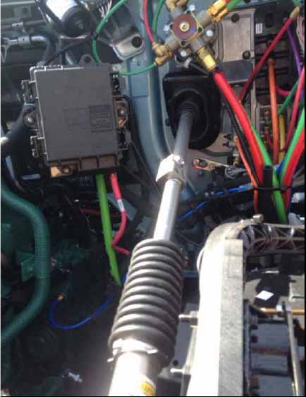
Two piece shaft design
