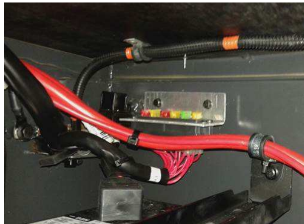
FIGURE 4 : For vehicles equipped with I-START dual battery system (from 3CET2V220G5177311 ), find K918 at the starter batteries compartment.
