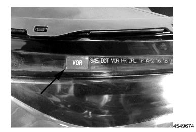
**4.** Peel the "VOR" label off of the backing paper and place it approximately 3mm inboard of the existing identification information. Repeat this process on both headlamps.
