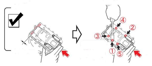
10. Tighten 5 nuts evenly in several increments in the order shown above using a socket driver while pushing the inflator and plate. (You will encounter some resistance during tightening because these nuts are self-locking nuts.). Torque: 3.9 N\*m (40 kgf\*cm, 35 in.\*lbf).
