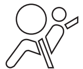
SRS Warning Light
