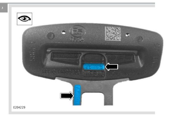
Record the seatbelt production date **AND** production part number on the repair order.
