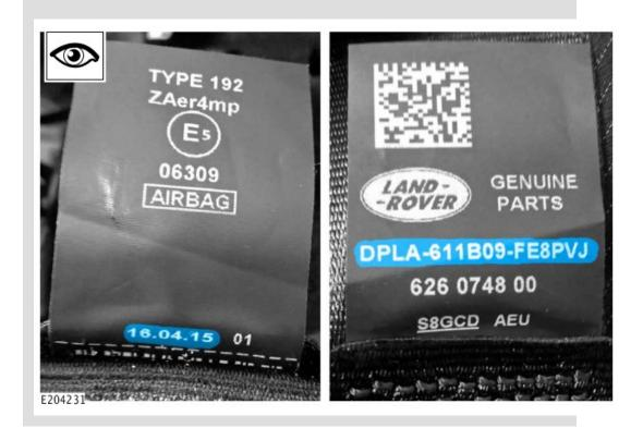
Record the front row seating left seatbelt production date **AND** production part number on the repair order.
