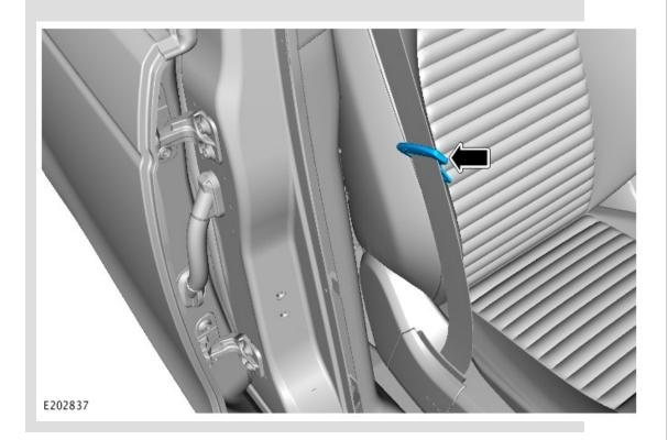
Locate the date embossed into the front row seating right seatbelt anchor.
