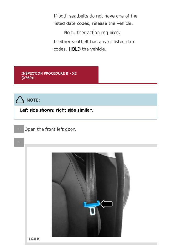
Locate the date embossed into the front row seating left seatbelt anchor.
