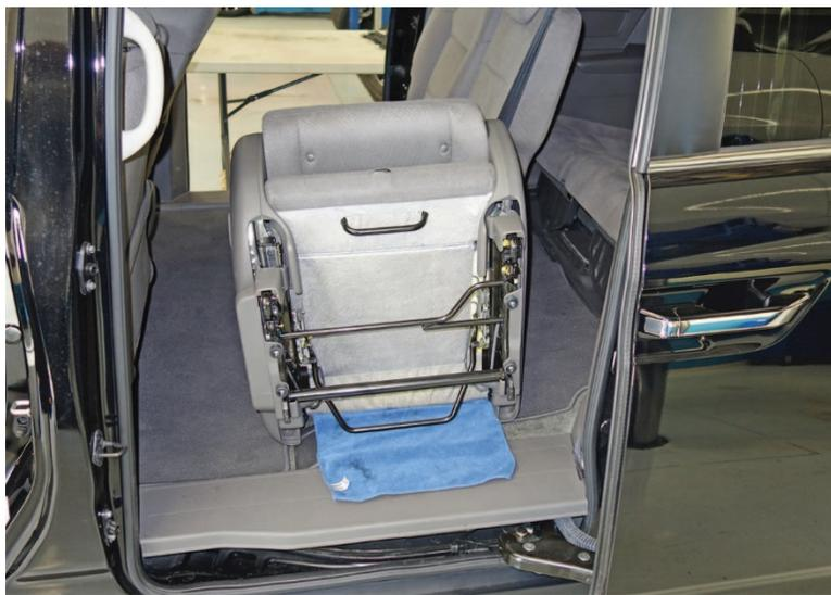
3. Remove the 12 mm nut located on the back of the seat rail (left side second row outer slide rail shown, others are similar).
