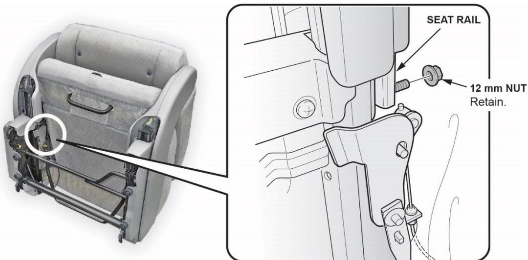
4. Install a bracket from the kit over the stud shown. Make sure the hook part of the bracket faces the back of the seat and the anti-rotation tab contacts the seat rail.
