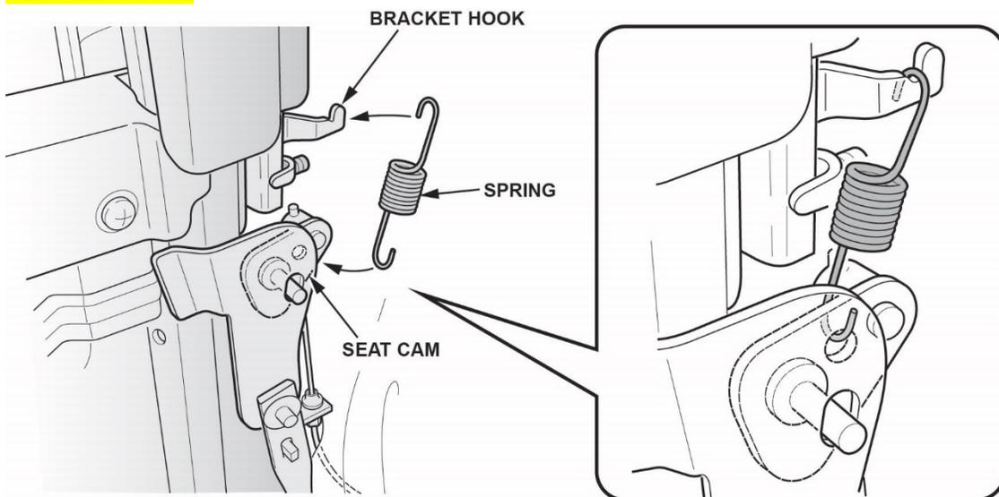
7. Install the other end of the spring onto the bracket hook as shown.
