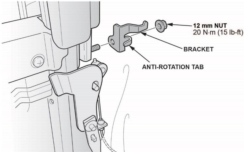
5. Reinstall the original 12 mm nut using a 3/8 in. flexible head torque wrench. Torque the nut to **20 N·m (15 lb-ft)**.
