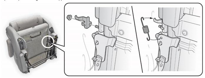
10. Install the second row seats in either the inner position (standard mode) or outer position (wide mode). First, hook the front part of the seat to the floor, then either push the seat toward the middle seat (standard mode) or pull the seat toward the door sill (wide mode) as shown below.
