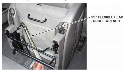
7. Install the spring from the kit through the back of the seat cam as shown.
