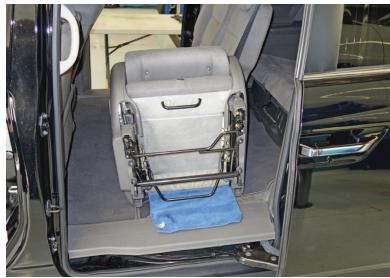
4. Remove the 12 mm nut located on the back of the seat rail (left side second row outer slide rail shown, others are similar).
