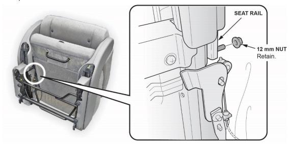
5. Install a bracket from the kit over the stud shown. Make sure the hook part of the bracket faces the back of the seat and the anti-rotation tab contacts the seat rail.
