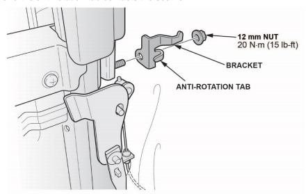
6. Reinstall the original 12 mm nut using a 3/8 in. flexible head torque wrench. Torque the nut to 20 N-m (15 lb-ft).
