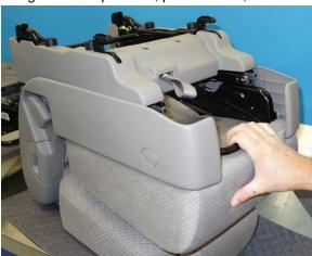
3. Using the seat slide lever adjuster and a feeler gauge, bend the slide lever to create 0.5 mm of space between the lever and the bracket as shown.
