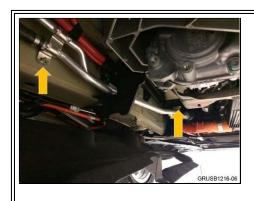
6. Check that the M6 bolt (DME ground connection "**Z6000\*4B**") is torqued to **8 Nm** as shown below and described in the repair instruction:
