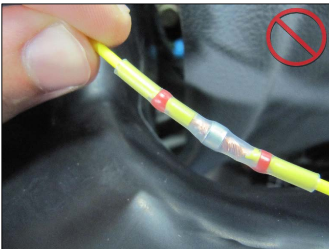
Unacceptable – Inadequate heat. Contour of the solder ring is clearly visible.
