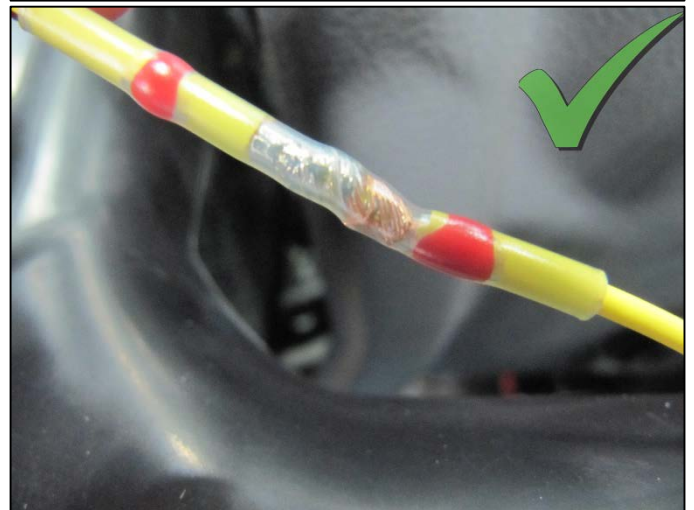
Acceptable – Solder is fully melted and sleeve has contracted.
