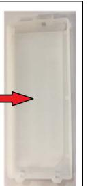
b. Apply the yellow warning label (from the parts kit) to the inside of the Junction Block fuse cover.
