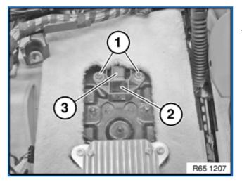
Unscrew nuts (1). Tightening torque <u>65 77 5AZ</u>. Remove sensor (2). Unlock plug connection (3) and disconnect. *Installation:* Make sure sensor is mounted without play.
