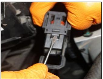
5. Using the correct new cover (Refer to the parts information on page 5: Based on the production range, two different covers are used. Select the one that matches the original.) re-assemble the connector in the reverse order of disassembly.
