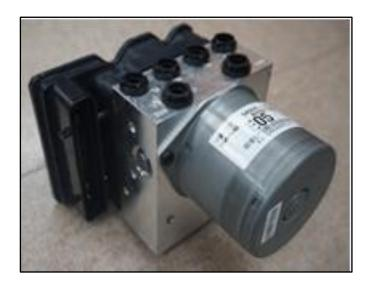
Mark HECU lines prior to removing the HECU and document for future reference to avoid incorrect re-assembly.
