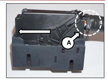
4. Press tab to release, remove, and discard the old connector cover.
