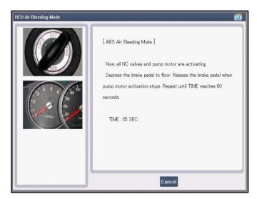
11. Once the test is completed as indicated on the screen, remove GDS/KDS.
