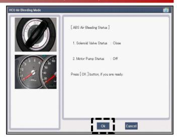
Follow instructions on screen except keep pedal depressed until test cycle completed message shows.
