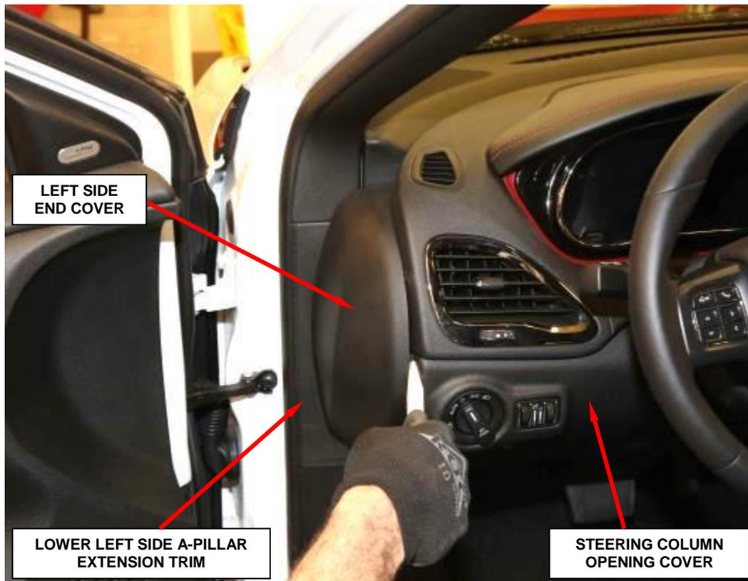
**Figure 4 – Left Side End Cover**
