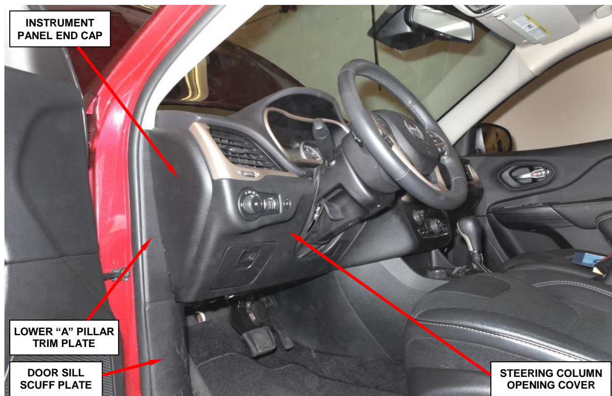
Figure 1 – Knee Airbag Steering Column Opening Cover
