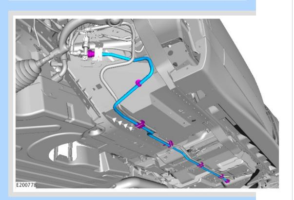
Remove and discard the fuel pipe assembly.
