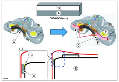
a. Clean the fuel tank where the pad will be attached (A).
