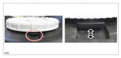
d. Replace the Main Fuel Pump assembly (B), retainer and gasket with new ones.
