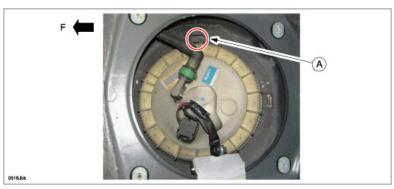
3. While keeping the alignment mark and the retainer notch aligned, tighten the fuel pump ring to the rotation angle (50-140 degrees) and specified torque (80-135 Nm, 8.2-13.7 kgfm, 59-99 ft lbf) using the SST. Total angle for step 2 and step 3 is 410-500 degrees: One full rotation (A) and tighten so the start position (3 ribs) comes to the star mark (B) using the SST (F=front of vehicle).
