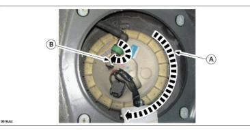
9. Attach two heat insulation pads (A) with tape (B) to the fuel tank (E) on either side (D) of the existing pad (C).
