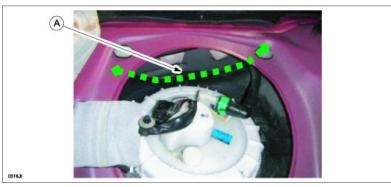
b. Remove the backing tape and attach the pad to the fuel tank as shown.
