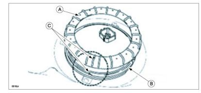
d. Install the modified fuel pump ring with the same procedure as the main side (aligning the positions of the fuel pump ring (A) and retainer (B) as shown (C).
