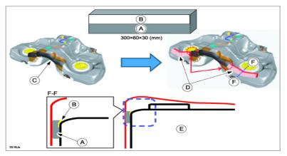
a. Clean the fuel tank where the pad will be attached (A).
