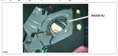
NOTE: Fit the groove of the SST into the rib of the fuel pump ring.
