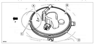
2. Align the positions of the retainer (A) and fuel pump ring (B) as shown (C), and tighten them one full rotation by hand.
