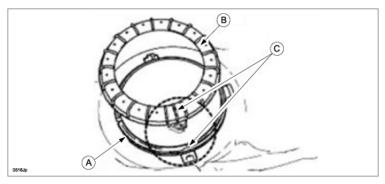
**NOTE:** If the retainer and fuel pump ring cannot be tightened by hand, remove the fuel pump ring, verify that there is no damage or misalignment on the retainer and fuel pump ring, and then tighten again.
