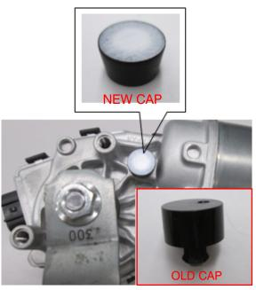
13. Verify that the new wiper motor has a breathing hole cap with a water proof cloth, as illustrated.
