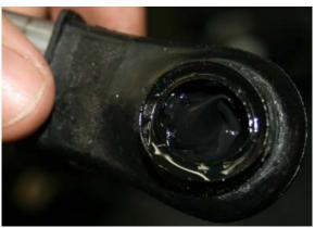
16. Fill the wiper link rod joint's resin cap with Multipurpose grease MZ100915EX (SAE J310, NLGI No. 2 or equivalent).
