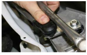
18. Connect wiper link rod to wiper motor link plate.
