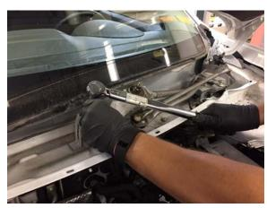
17. Bolt wiper motor and link assembly to vehicle.
