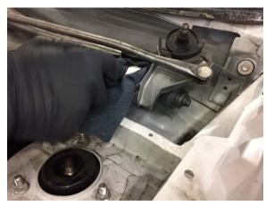
8. Separate the wiper link rod joint from wiper motor link plate.
