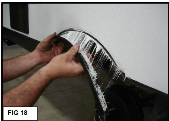
10 Fig 18: Pull the wheel well trim off of both sides of the trailer.
