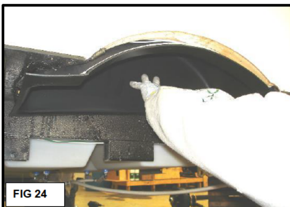
13 Fig 24: Put the new wheel well up inside the opening of the trailer. Any wiring should be tucked up above the wheel well as you put it in place.
