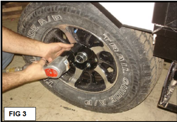
2 Fig 3: Remove all lugs on both wheels. Use the impact driver and 13/16" impact socket. Remove both wheels from axle.
