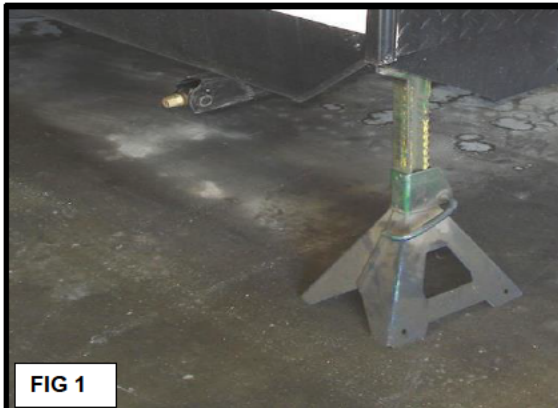
1 Fig 1: Raise the trailer using jackstands. Wheels should be completely off the ground.
