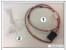
Repair kit overview: Repair harness (1) Butt connector and shrink tubing (2)
