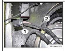
Repair harness procedure: Locate the fuel pump electrical connector (1). Unwrap the tape (2) from rubber grommet.
