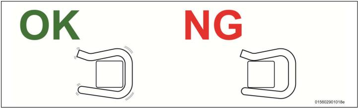
Note: When correctly installed the clip will wobble. If not fully installed there will be no play in the clip.
