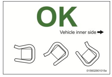
b) Ensure that the clip is fully engaged.
