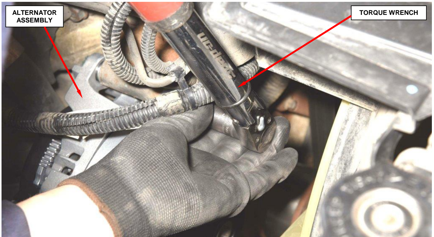
Figure 7 – Tighten Mounting Bolts to Specifications
