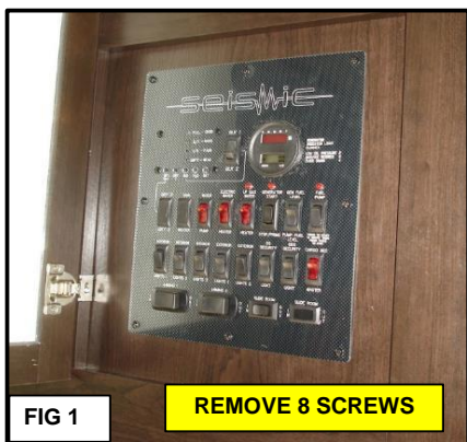
1 Fig 1: Remove 8 screws from the Command Center Panel with the screwgun and #2 square bit.
