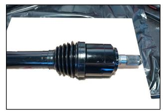
15. Place the smaller boot band (K) installed in step 9 onto the boot and secure using **SST 09495 3K000**.
