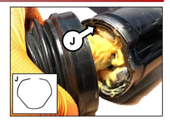
14. Attach the tripod boot to the tripod housing.
