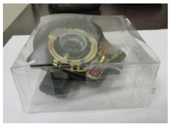
**NOTE:** The new wiper motor cover is prepackaged with butyl rubber and grease. Be extremely careful when removing it from the package and when handling. Do not touch the grease or butyl rubber. The new cover also has a yellow paint mark for identification as shown in the installation photos below.
