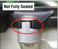
15) Connect wiper motor wiring connector.
