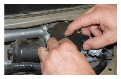
13) Using the order below, loosely install the screws. Continue tightening the screws sequentially, a little at a time, to seat the cover.
