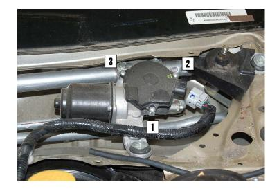
14) Torque screws to 2.0 N•m (17.2 in-lb) in the above order. Check to make sure there are no gaps indicating the wiper motor bottom cover is fully seated.
