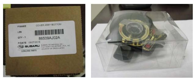
**NOTE:** The new wiper motor cover is prepackaged with butyl rubber and grease. Be extremely careful when removing it from the package and when handling. Do not touch the grease or butyl rubber. The new cover also has a yellow paint mark for identification as shown in the installation photos below.
