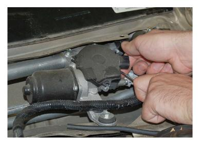
9) Lift up the right side of the wiper motor bottom cover with one hand and carefully using a flat-head screwdriver or plastic tool in the other, disengage the terminal from the terminal socket. Remove wiper motor bottom cover by pulling straight up from both sides.
