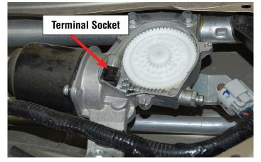
**IMPORTANT:** Make sure there is no butyl rubber in the terminal socket. If present, the wiper motor will not operate.
