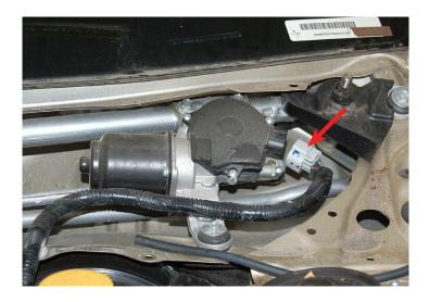
7) Using a magnetized #2 Phillips-head screwdriver, remove the 3 screws from the wiper motor bottom cover in the following order.
