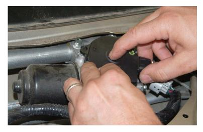
13) Using the order below, loosely install the screws. Continue tightening the screws sequentially, a little at a time, to seat the cover.
