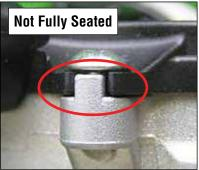
15) Connect wiper motor wiring connector.
