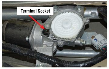
**IMPORTANT:** Make sure there is no butyl rubber in the terminal socket. If present, the wiper motor will not operate.
