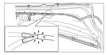
6) CAREFULLY disconnect wiring harness connector from wiper motor.
