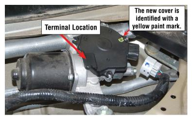
12) Press down the wiper motor bottom cover gently and evenly over the terminal location to insure that the terminal is properly seated in the terminal socket.
