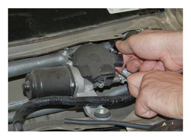
9) Lift up the right side of the wiper motor bottom cover with one hand and carefully using a flat-head screwdriver or plastic tool in the other, disengage the terminal from the terminal socket. Remove wiper motor bottom cover by pulling straight up from both sides.
