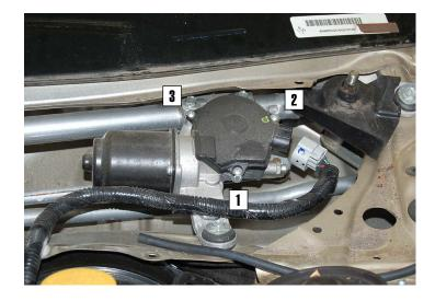
14) Torque screws to 2.0 N•m (17.2 in-lb) in the above order. Check to make sure there are no gaps indicating the wiper motor bottom cover is fully seated.
