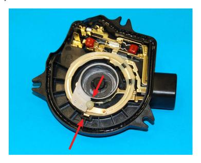
**IMPORTANT NOTE:** Make sure that the relay joint plate is in the correct position prior to installing the wiper motor bottom cover. This will ensure proper fit during installation and alignment.
