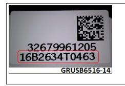
Before installing the replacement part, the new air bag module's serial number must be documented by the technician on the repair order so it can also be entered into the warranty claim's comment section.
