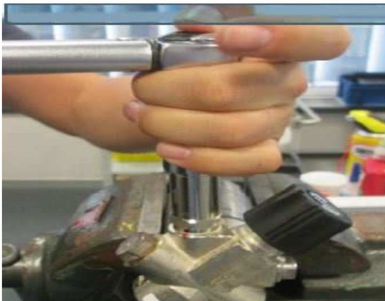
Figure 8: Torque PRD to 26 FT-LBS
