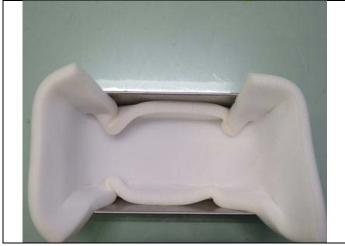
a) Place the polyurethane in the center of the steel case.
