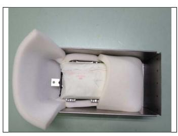
c) Fold over the urethane as shown and tuck the urethane between the air bag and the case.
