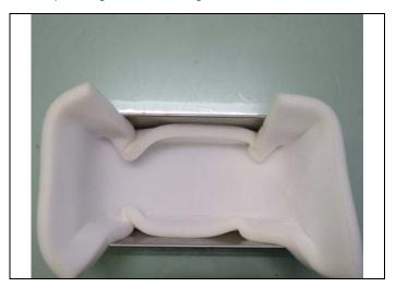
a) Place the polyurethane in the center of the steel case.
